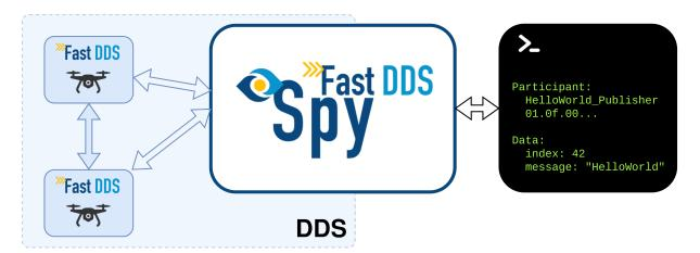
eProsima Fast DDS Spy is easily configurable and installed with a default setup, so that DDS topics, data types and entities are automatically discovered without the need to specify the types of data. This is because this tool exploits the
