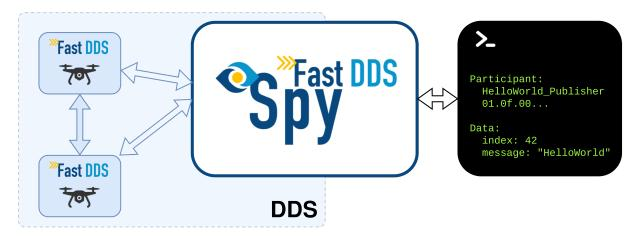
*eProsima Fast DDS Spy* is easily configurable and installed with a default setup, so that DDS topics, data types and entities are automatically discovered without the need to specify the types of data. This is because this tool exploits the DynamicTypes functionality of eProsima Fast DDS, the C++ implementation of the DDS (Data Distribution Service) Specification defined by the Object Management Group (OMG).
